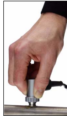
Wall thickness measurement
