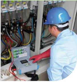
MicroOhm MI 3250 is portable low resistance ohmmeter for measuring low resistances of breakers and switches, busbars, cable joints, small to medium sized transformer and motor windings for industrial application, etc., with test current up to 10 A.
