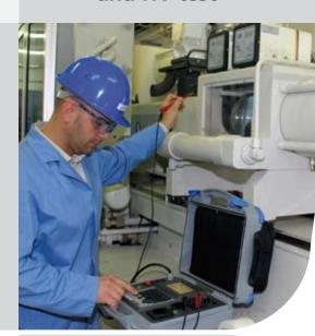
Multifunctional portable test instrument MultiservicerXA is intended to perform all necessary measurements for testing the electrical safety of portable electrical equipment, machines and switchgears.
