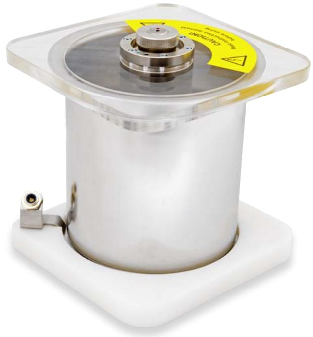
The CP TC12 is used in conjunction with the CPC 100 and CP TD1 to measure tangent delta / power factor and permittivity of insulation liquids, e.g. transformer oil. The three-electrode design with guard allows precise measurement, especially of small losses.
