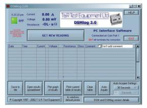
Connecting the DSM200 to a PC running the optional DSM/og software adds data capture and reporting functions to the unit, allowing test results to be exported directly to Excel or saved to a file. All results are time stamped, and a comment may be added to each test. Data capture can be controlled from the PC, and the resistance of a test object can be monitored over a period of time.
