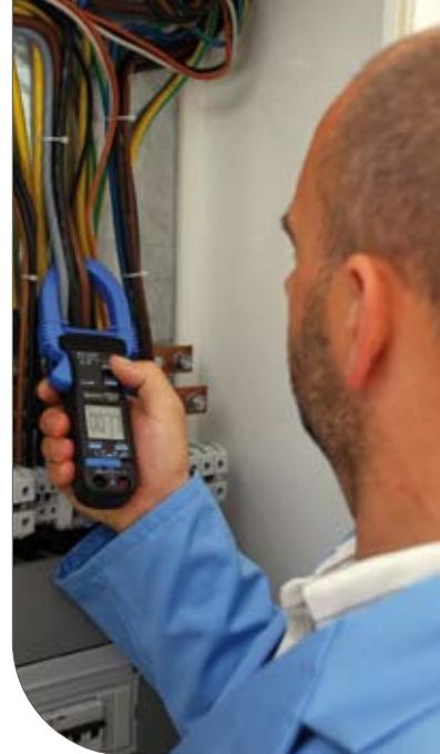
**MD 9220**, the professional current clamp with TRMS measurement and wide jaw opening, enables current measurement up to 2000 A. This current clamp, using state-of-the-art measurement technology and housed in a sturdy industrial-grade case, represents the ideal choice for the works electrician.
